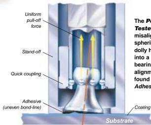
The **PosiTest Adhesion Tester** compensates for misalignment. The uniquely spherical articulating dolly head is engaged into a ring of small ball bearings, ensuring correct alignment. This feature is found only on the **PosiTest Adhesion Tester**.
